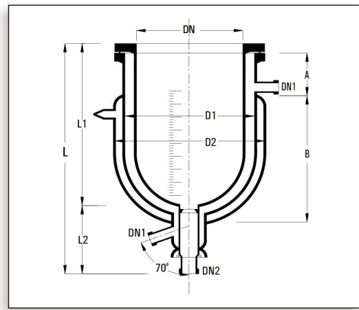
Goel is presenting Flexi (Detachable) "Transparent Double Jacketed Vessel" to maintain the leading position in industry by way of developing indigenously newer products with higher value towards their Mission and to cater the customer via innovation.
