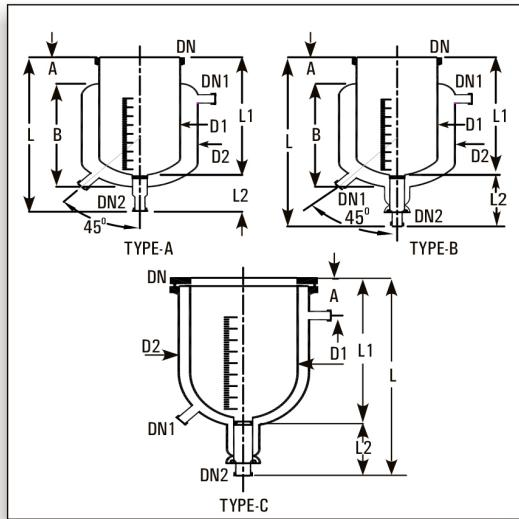
For special applications, cylindrical vessels can be supplied with a jacket for heating or cooling. Jacket is sealed to the vessel with Viton 'O' ring and other sealing compositions. The seal prevents high stresses between vessel and jacket by allowing the movement flexibility between two due to thermal expansion.
