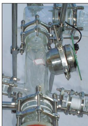
Electro-magnets are used to operate Magnetically operated Reflux dividers. When 'On' the magnet attracts the swinging funnel of the reflux divider so that distillate can be taken off.
