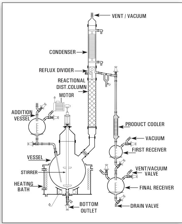
This is a versatile unit and can be used as Reaction Distillation Unit, Fractional Distillation Unit or a combination of both. All features of Reaction Distillation Unit and Fractional Distillation Unit are incorporated.
