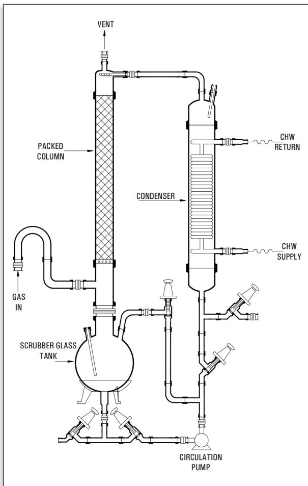
Goel offer Pilot Plant Gas Scrubber for various gases like HCl, Cl<sub>2</sub>, SO<sub>2</sub>, Br<sub>2</sub>, HBr, NO<sub>x</sub> etc or any other corrosive gases. These scrubbers use the media as water / Aq. NaOH / any other suitable solvent which can neutralise the exhaust gases. Our Pilot plant scrubber are ranging from 20L vessel capacity to 500L vessel capacity and scrubber diameter from 80DN to 300DN.
