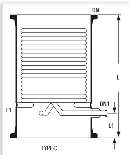
Condensers are used for condensation of vapours and cooling of liquids. Condensers are made by fusing number of parallel coils in a glass shell. Coils are made in different diameters using tubes of different bores.
