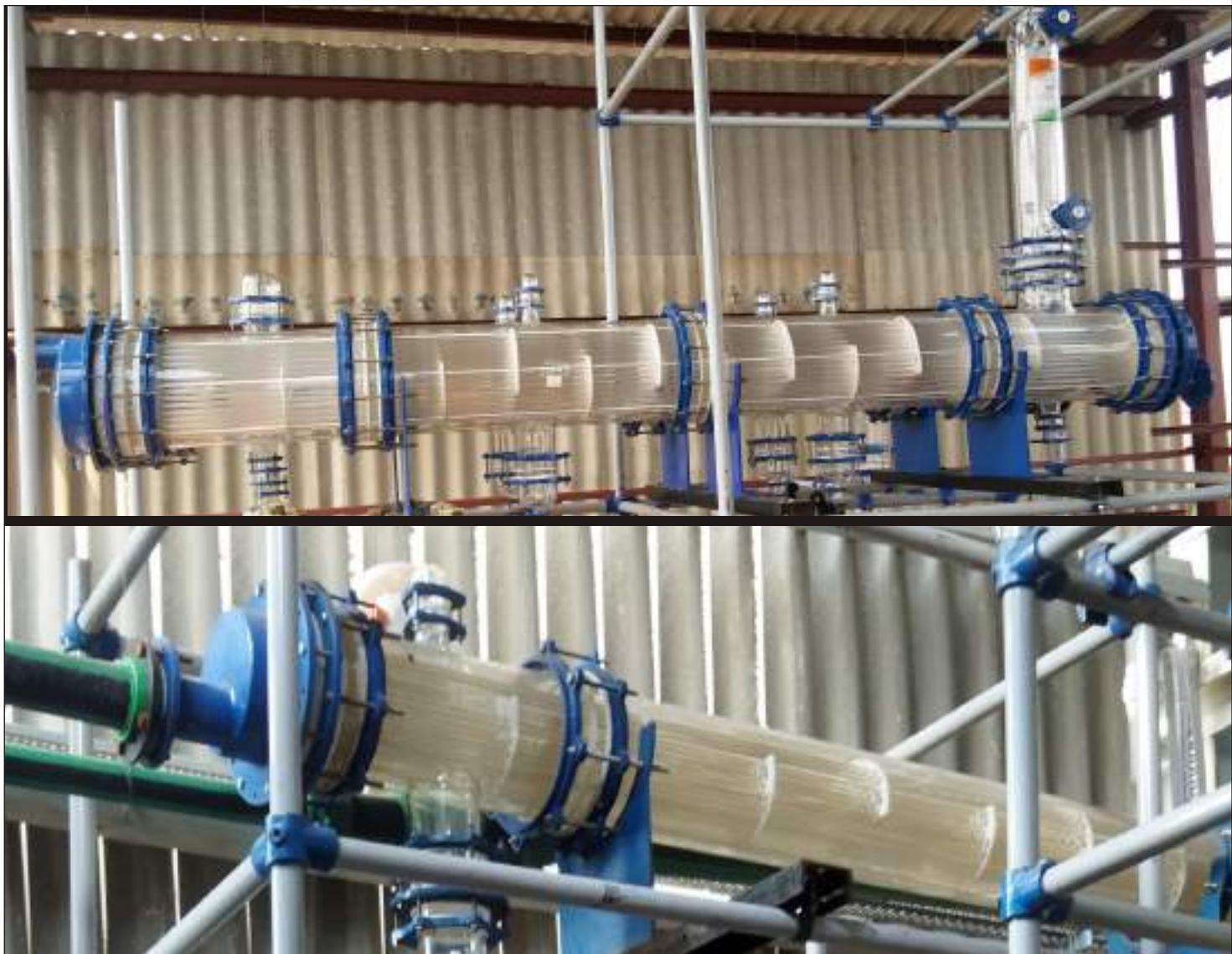
The overall heat transfer co-efficient of Borosilicate glass equipment is comparatively favourable with many alternative materials because of its smooth surface which improves the thermal coefficient & reduce the tendency of fouling.
